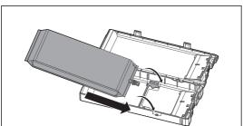
If you are using 2L ink bag, release the lock of divider plate in the case, and then put the ink bag into the case.
