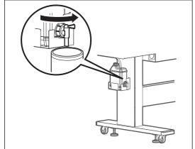
Open the waste fluid valve, and transfer the waste fluid to the container.
