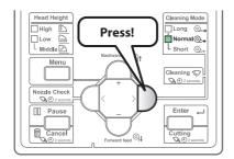
Press the [Cleaning] key, so that the "Normal" indicator (one of the "Cleaning Mode" indicators) lights steady.
