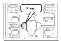
Press the [Nozzle Check] key for more than two seconds.
