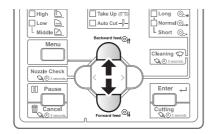
Press the [Forward] key or the [Backward] key on Operation panel.
