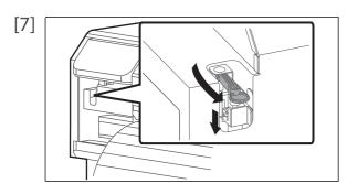
Press the tab of Cutter lightly, return Cutter holder to its initial position.
