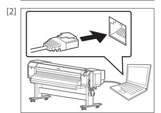
Connect the Gigabit Ethernet cable to the computer.
