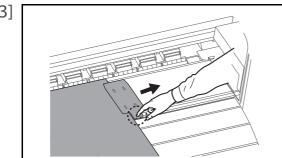
While keep pressing the part circled with a dotted line in the figure left, slide the media holder to the right to remove it from the media.
