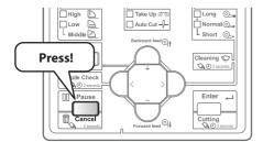
Press and hold the operation key on the operation panel for two seconds or more during printing.
