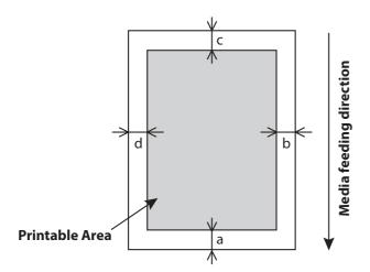
a=5 mm \*1 b=5 mm to 25 mm c=5 mm d=5 mm to 25 mm
