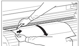
Pull the media towards you, and cut the torn part with cutting tools such as a razor blade.
