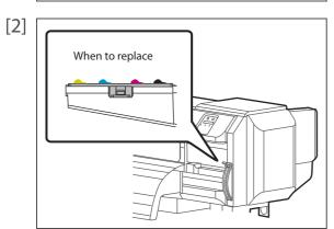
Check the absorption material for the flushing box.
