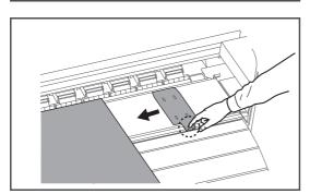
Keep the part circled with a dotted line in the figure to the left pressed to set the media holder.
