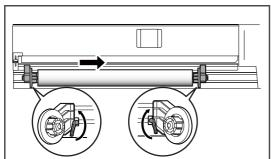
Loosen the Fixing levers of the right and left Roll media holders, move the roll media to the center.
