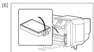
Pull the tab up of the absorption material for the flushing box, and release the hook.
