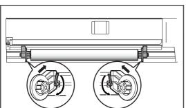
Press Roll media holder toward the printer and fix the Fixing levers.
