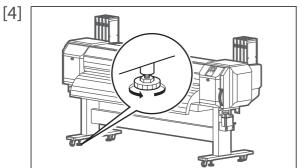
Loosen the four adjusters of Stand as shown in the left.
