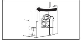
After pouring the waste fluid to the empty container, close the waste fluid valve securely.
