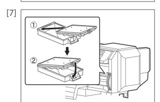
Attach new absorption material for the flushing box.
