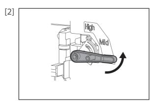
Change the head height by moving Head height adjustment lever (orange).
