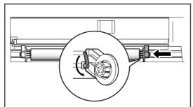
Attach Roll media holder (right) to the roll media and tighten Fixing
