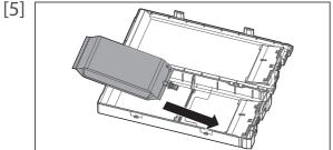
If you are using 2L ink bag, release the lock of divider plate in the case, and then put the ink bag into the case.
