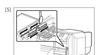
Wipe the right side surface of the base of cleaning wiper going back and forth.
