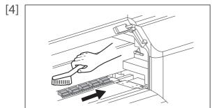
Brush off dusts on the pressurizing rollers with a soft brush.
