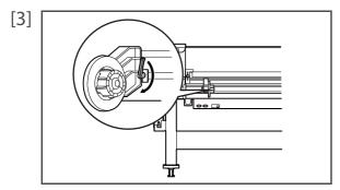
Tighten Fixing lever of Roll media holder (left) and fix the Roll media holder (left).
