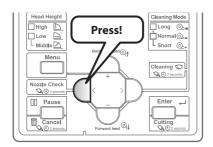
Press the [Nozzle Check] key for more than two seconds.
