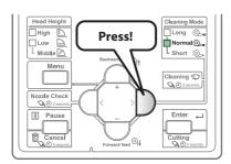
Press the [Cleaning] key for more than two seconds.
