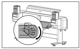
Rewind the roll media a little by rolling Flange on Roll media holder while holding the edge of the media, and eliminate any slack or slant.
