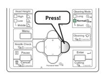
Press the [Cleaning] key for more than two seconds.
