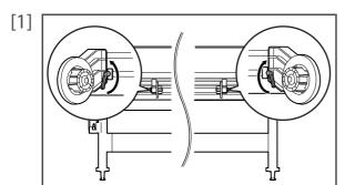
Loosen Fixing levers on the Roll media holders (both left and right) on the back of the printer.
