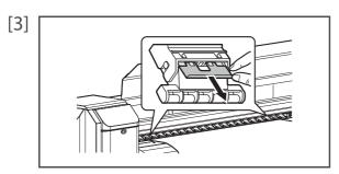
Release the pressurizing rollers on both edges of media.
